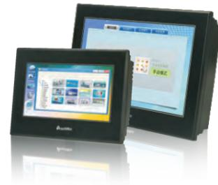
Oil proof model with suffix P re-design the cover and film. The film back adhesive tape width increased to prevent from the oil. Other functions are the same. The models are fit for the heavy oil environment.
