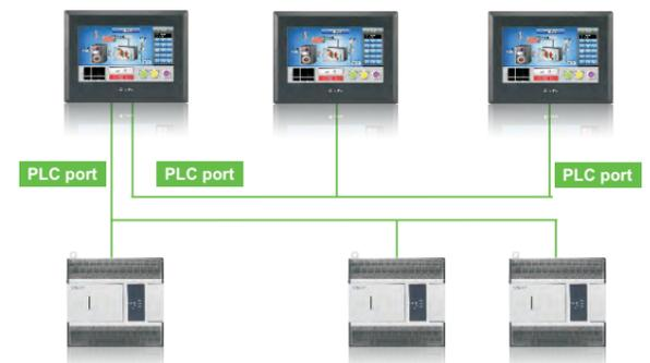
**Pass through function, remote upload and download program via HMI, monitor the PLC state**
